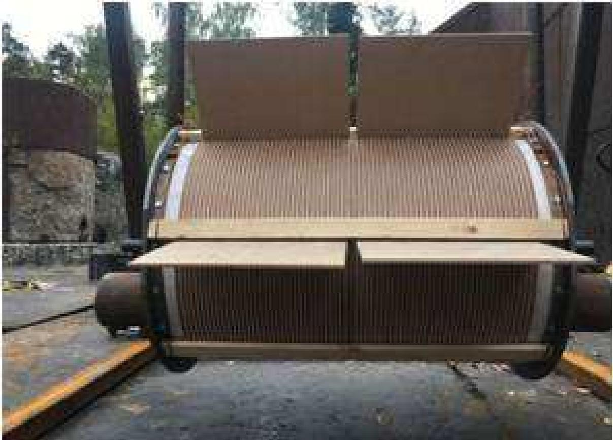
**Figure 2.** Fiberglass construction test: the shell with explosive device in ballistic pendulum.
