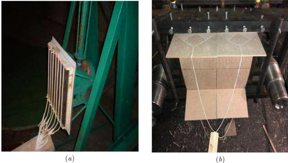
**Figure 1.** Gasdynamic devices for generation of low-impulsive loads: (a) tape explosive charge; (b) controlled initiation explosive charge.
