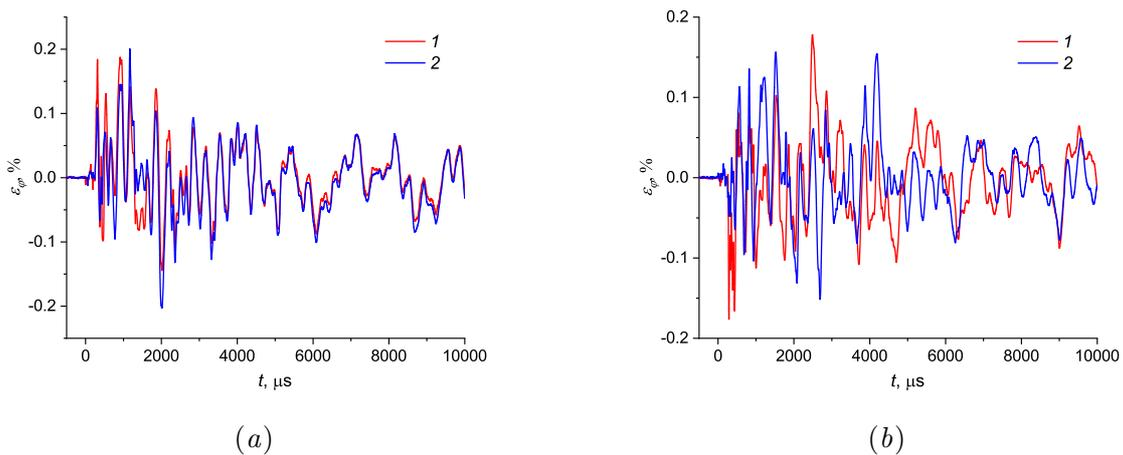
**Figure 3.** Fiberglass construction test: (a) comparison of circular deformations at  $\varphi = 0^\circ$  measured by the KB-10-200 (1) and BF350-3AA (2) strain sensors; (b) circular deformations vs time  $t$ ,  $\varphi = 90^\circ$  (1) and  $180^\circ$  (2).
